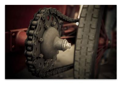
\*The advantage of a chain drive that uses sprocket gears over using spur gears is the ability to transfer torque and speed over longer distances.
