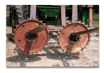
Sprocket gears have more space between their teeth in order for a chain to fit in between them.
